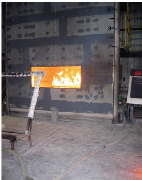
Wall is built with ProGUARD® applied to outside and sealed. Interior room is lit on fire.
