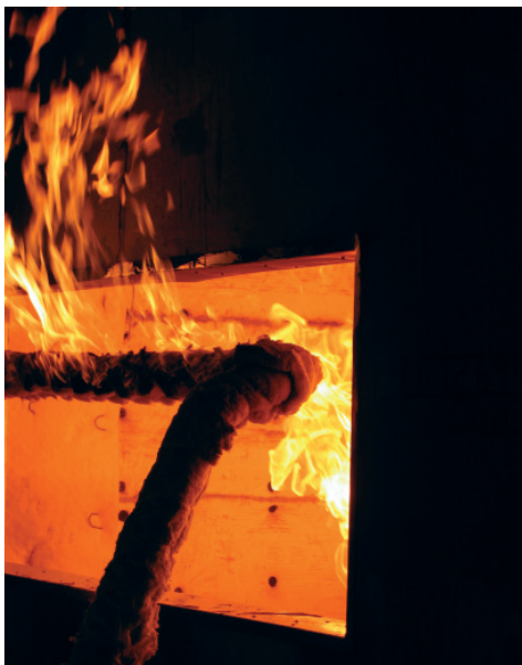
Flame is placed beneath window cutout in wall as well.
