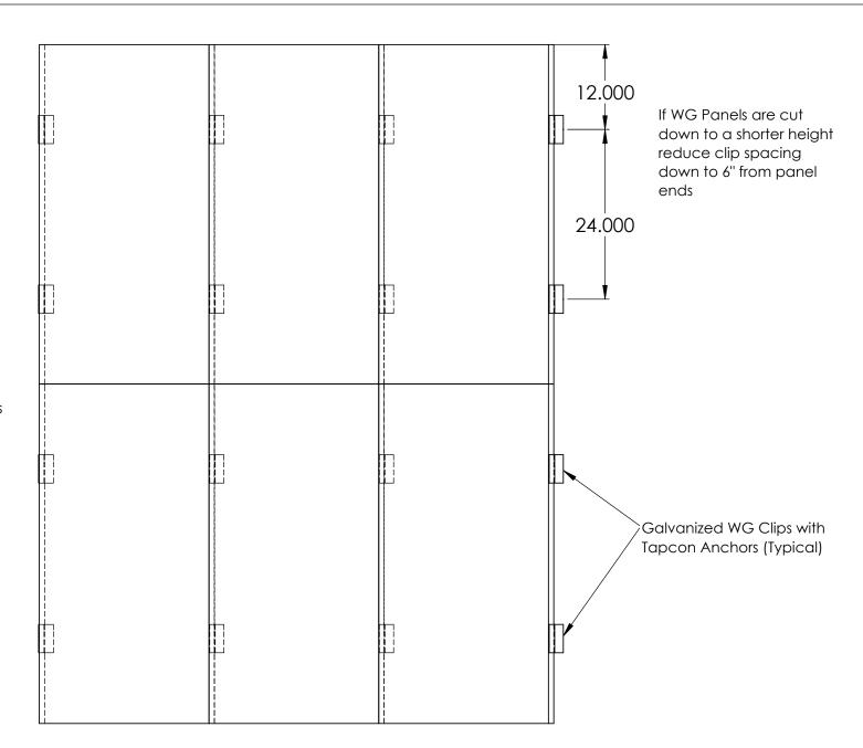
WG Panels are dry stacked, there is no requirement for caulking between stacked panels
